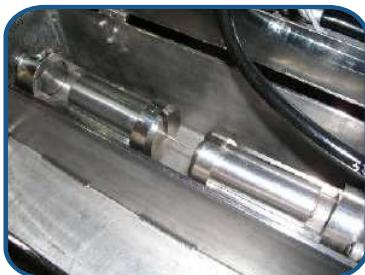
Hydraulic system used is a tension load cell with sensitive membrane.
